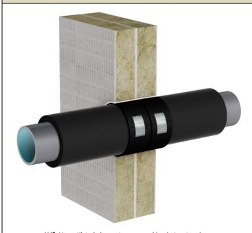
U/C: Unventilated pipe systems e.g. cold or hot water pipes. Plastic pipes can be at all angles between 90  $^{\circ}$  and 45  $^{\circ}$  relative to the wall.
