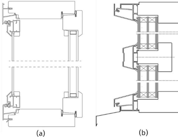
a) MSE 2+1 is an openable window composed of inner sash with a double-glazed insulating glass unit consisting of two 4 mm glasses, argon gas and double gaskets, and outer sash with a single 4 mm float glass and a single gasket. Both sashes have pin hinges and locks, and inner sash has metal hole covers.
