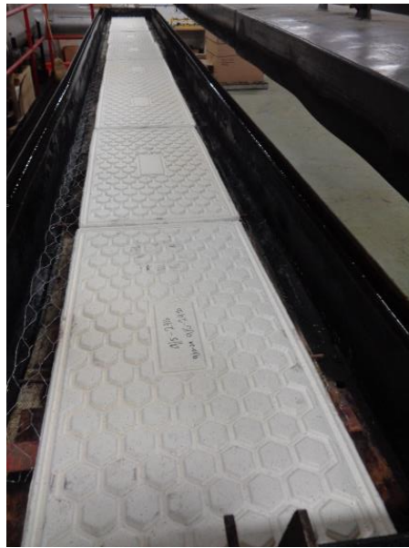
Photo No. 1 Unexposed Surface of the Test Specimen (Pre-test)
