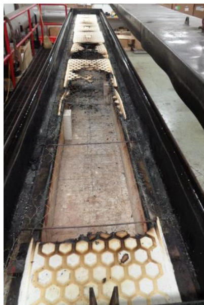
Photo No. 2 Unexposed Surface of the Test Specimen (Post-test)
