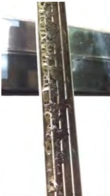
Figure 65: Coating has worn excessively, signs can include carbon dust on and inside rope
