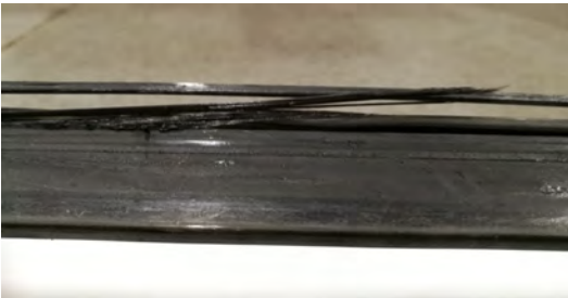
Figure 61: Local loss of load bearing material
