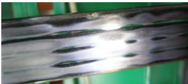
Figure 69: Normal surface wear pattern
