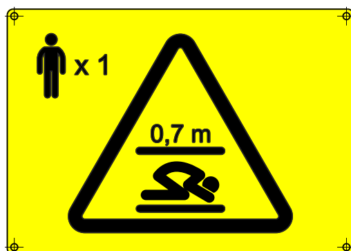
Figure 14: 0.7 m refuge space label in the pit
