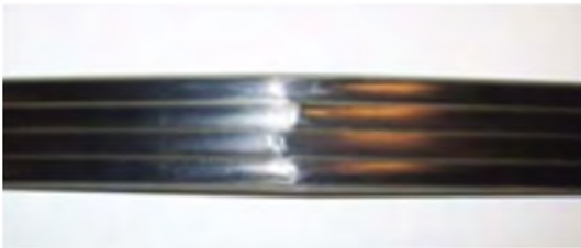
Figure 57: Transverse CFRP damage
