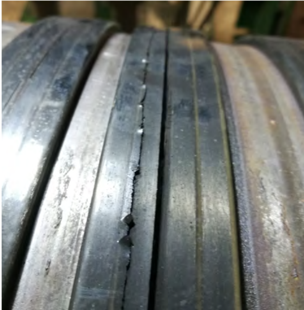
Figure 64: Crack penetrates whole thickness of rope
