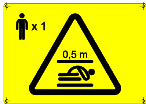
Figure 12: 0.5 m refuge space label in the pit
