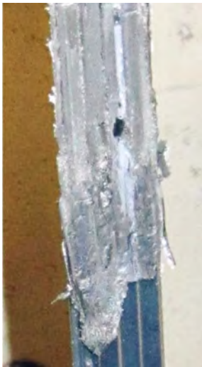
Figure 56: Coating has melted and CFRP has been damaged
