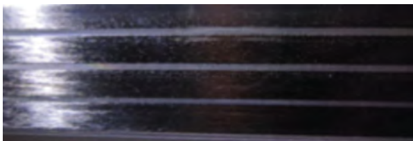
Figure 70: Small bubbles embedded in rope Possible cause: manufacturing.
