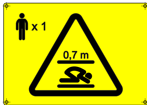
Figure 11: 0.7 m refuge space label in the pit
