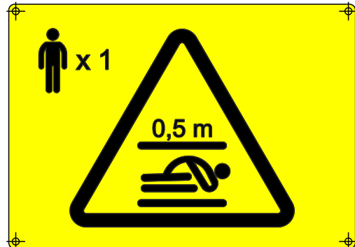
Figure 9: 0.5 m refuge space label in the pit
