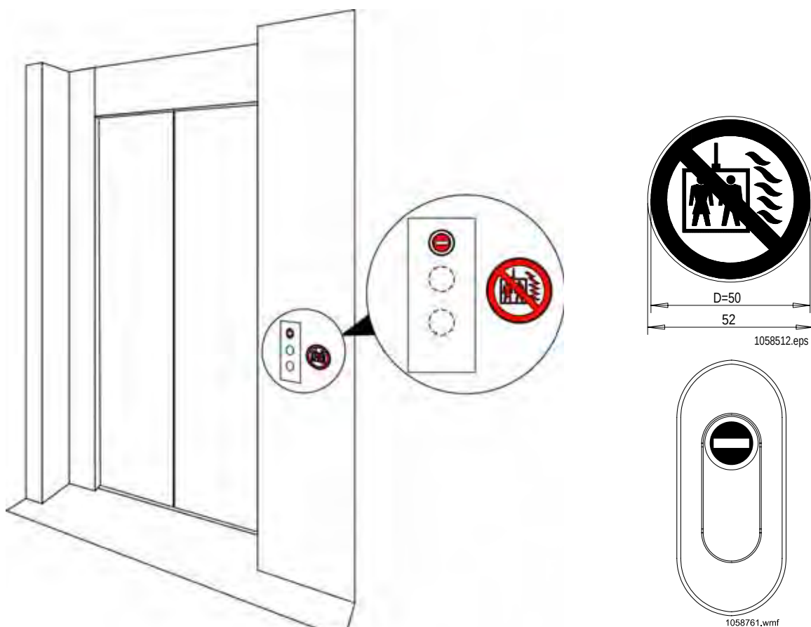
Figure 5. Elevator "No entry" indicators
