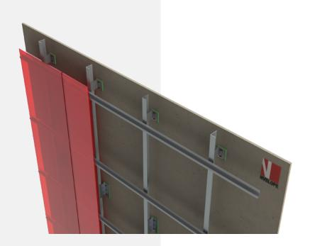
NVELOPE brackets are secured directly to a new or existing substrate of; concrete, brickwork or blockwork or steel frames. Suitable primary anchors are employed to position the brackets to a pre-determined grid to suit the Panel layout – please liaise directly with preferred NVELOPE Primary Fixing supplier re pull-out.
