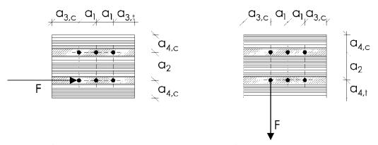
For screws in the edge surface,  $a_1$  and  $a_3$  are parallel to the CLT plane face,  $a_2$  and  $a_4$  perpendicular to CLT plane face.
