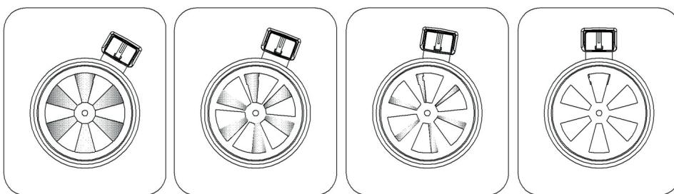
OPEN - HIGH TEMPERATURE ← → LOWER THE TEMPERATURE ← → CLOSED – EXTINGUISH
