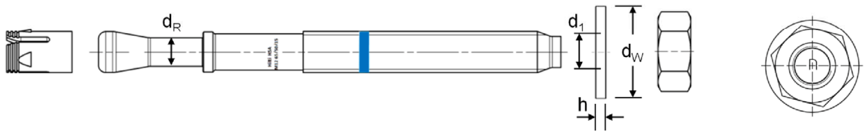
Figure A2: Hilti metal expansion anchor HSA-BW
