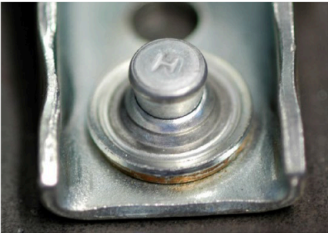
Clearly visible piston mark on top washer
