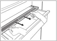
If you need to replace the device's white membrane, grab the device in the middle and separate the membrane from the cover by pulling the cover.
