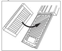
3. Hold the filter down while closing the plastic housing until you hear a click.
