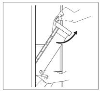
3. Lift and turn the drawer to pull it out of the appliance.
