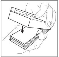
Remove the top glass shelf from the fridge compartment. Slip the plastic housing with the air filter on the left side of the glass shelf.
