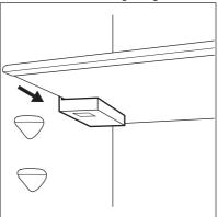
Replacing the air filter
