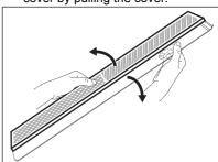
Assemble a new membrane into the cover by pressing the edge of the membrane into the cover.
