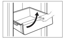
**3.** Pull the drawer out while lifting it up and detach it from the rails.
