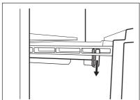
**3.** Pull the drawer out while lifting it up and detach it from the rails.
