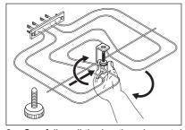
2. Carefully pull the heating element down.
