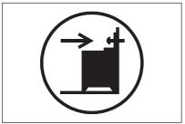
Install the anti-tilt protection B - 343 mm down from the top surface of the appliance and A - 67 mm from the side of the appliance into the circular hole on a bracket. Screw it into the solid material or use applicable reinforcement (wall).
