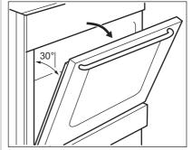
Hold the door trim (B) at the top edge of the door on both sides and push inwards to release the clip seal.
