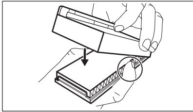
3. Remove the top glass shelf from the fridge compartment. Slip the plastic housing with the air filter on the left side of the glass shelf.
