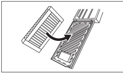
2. Hold the filter down while closing the plastic housing until you hear a click.
