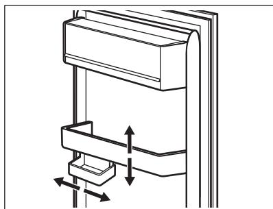
This model is equipped with a variable storage box.
