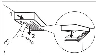
2. Remove the used air filter.
